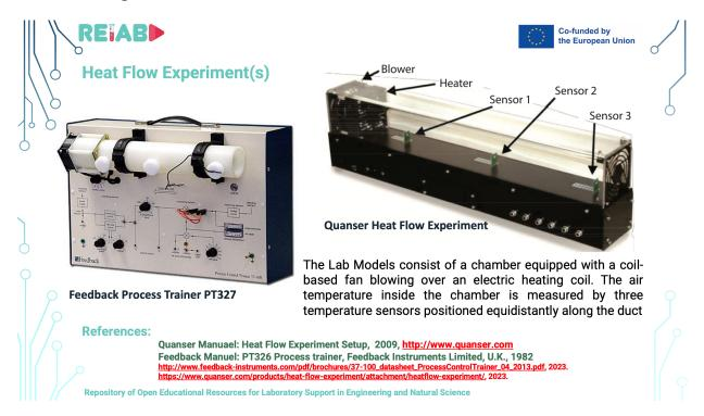
Heat flow experiments are based on following type of experimental setups 1) PT 326 Process Trainer, Feedback Instruments Limited, http://www.feedback-instruments.com, 2) Quanser Heat Flow Experiment, https://www.quanser.com, or 3) PT400 Laboratory Model, University of Kragujevac, with following general description
