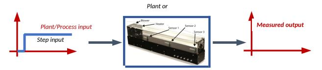
Input signal is step: 5+1\*h(t-11). Output signal is step response of the system in open loop. The sampling time is  $T_s = 0.11$  [s]. Environmental conditions are the same for all experiments. Conduction of experiments is going consequently with maximal pause about one minute.
