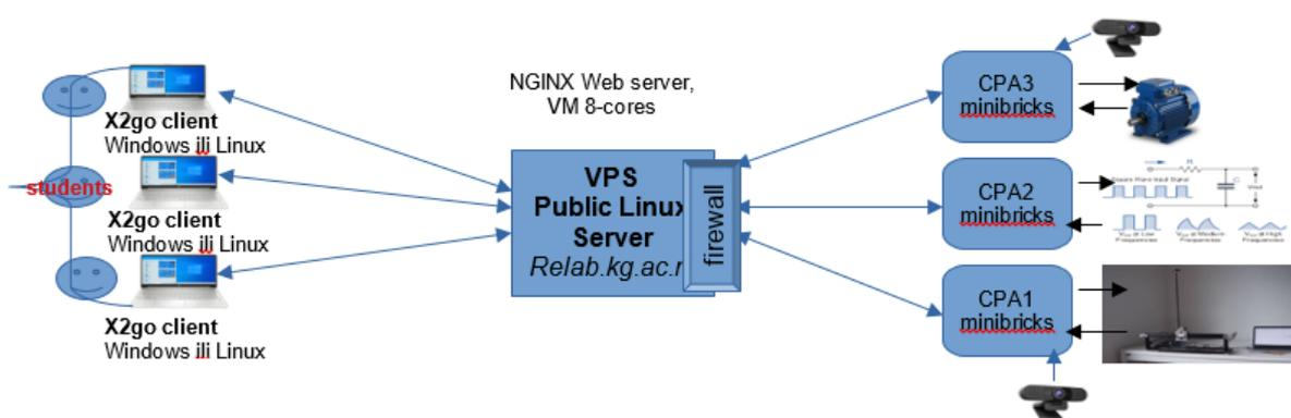
Fig 6. Configuration pilot installation of WEB Laboratory at University of Kragujevac
