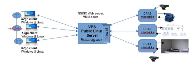
Fig 6. Configuration pilot installation of WEB Laboratory at University of Kragujevac
